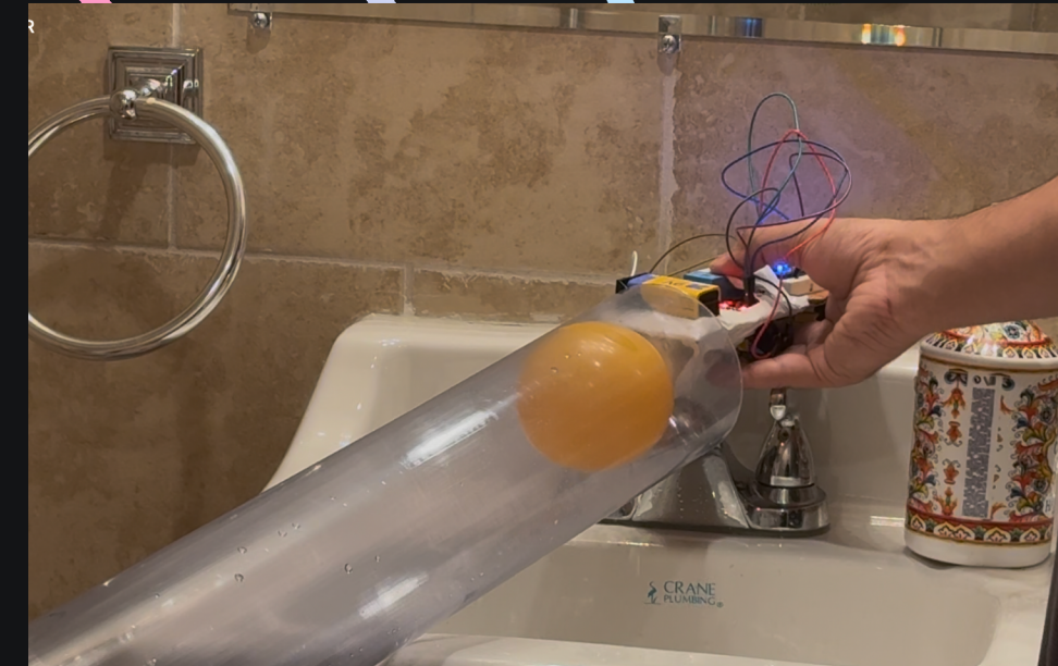
An O-Seal prototype in testing, inflating in a pipe and sealing up a crack.
