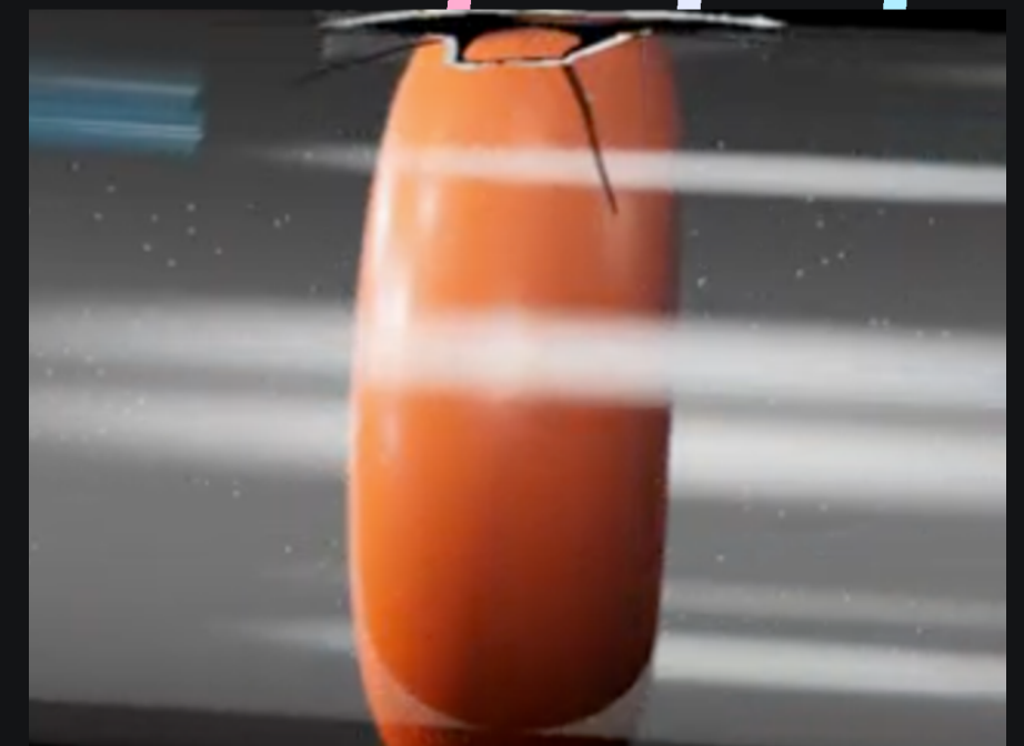
A simulation showing how an O-Seal expands and stops cracks, allowing water to flow through.
